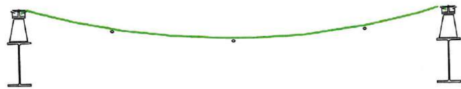
Figure 1—A sketch diagram of a one-foil, cable-supported ETFE system.
