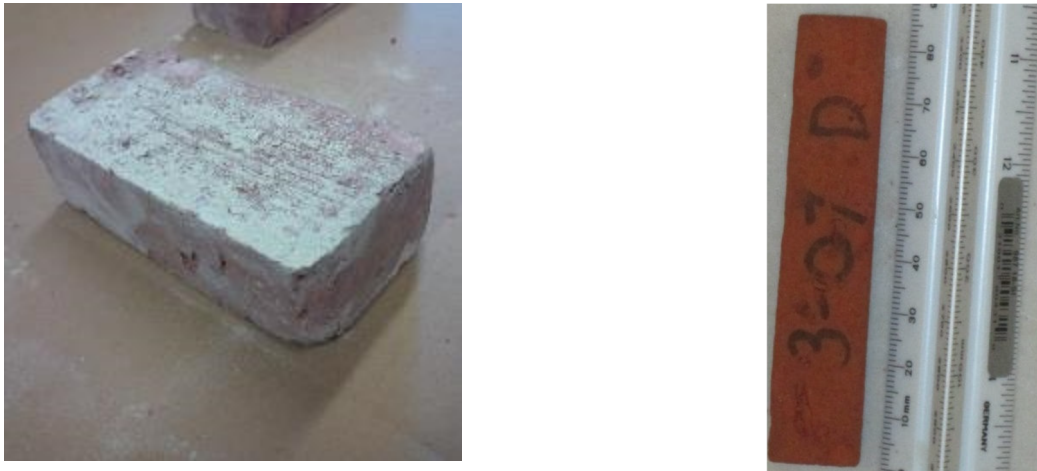
Figure 3. Full brick sample (left) and slice (right) for freeze-thaw testing for sample 3.
