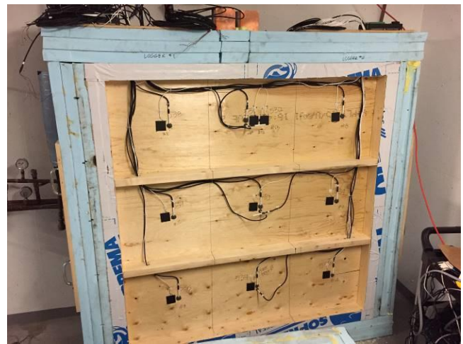
Figure 11 – Location of Heat Flux Sensors on Underside of Hot Lid
