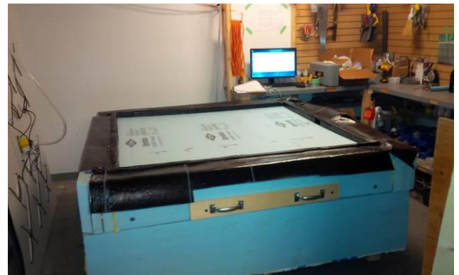
Figure 3 – Hot Box with Roof Insulation
