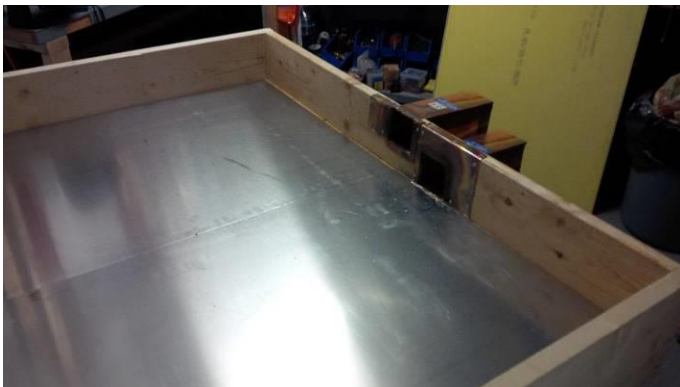
Figure 2 – Hot Box Aluminum Base
