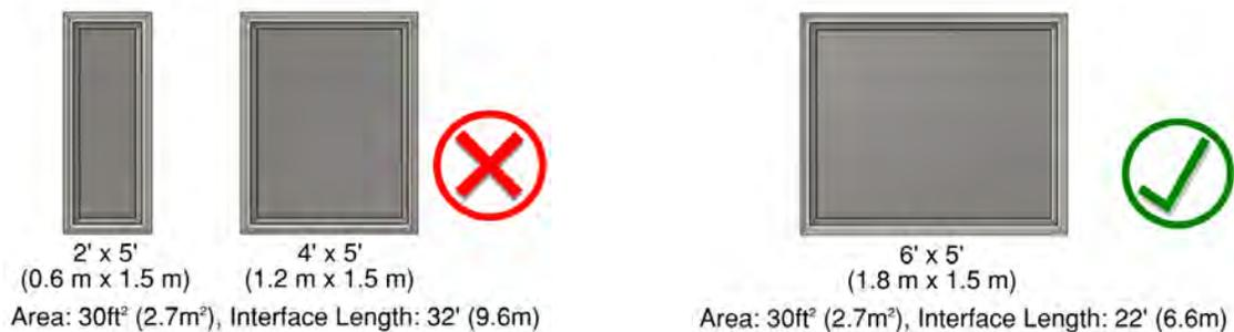
Minimizing the window perimeter and frame length by maximizing the size of glass per opening was introduced in Chapter 5 and is illustrated in the graphics above. **Figure 6.5** outlines the impact of glazing size on thermal transmittance and overall wall thickness for
