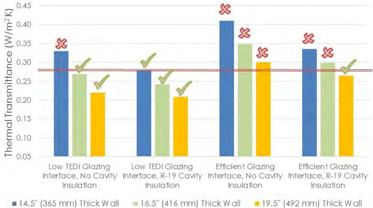
**Figure 6.2:** Impact of Window to Wall (Glazing) Interface Transmittance on Wall Thickness for a Target of 0.28 W/m<sup>2</sup>K (R-20 effective)<sup>1</sup>
