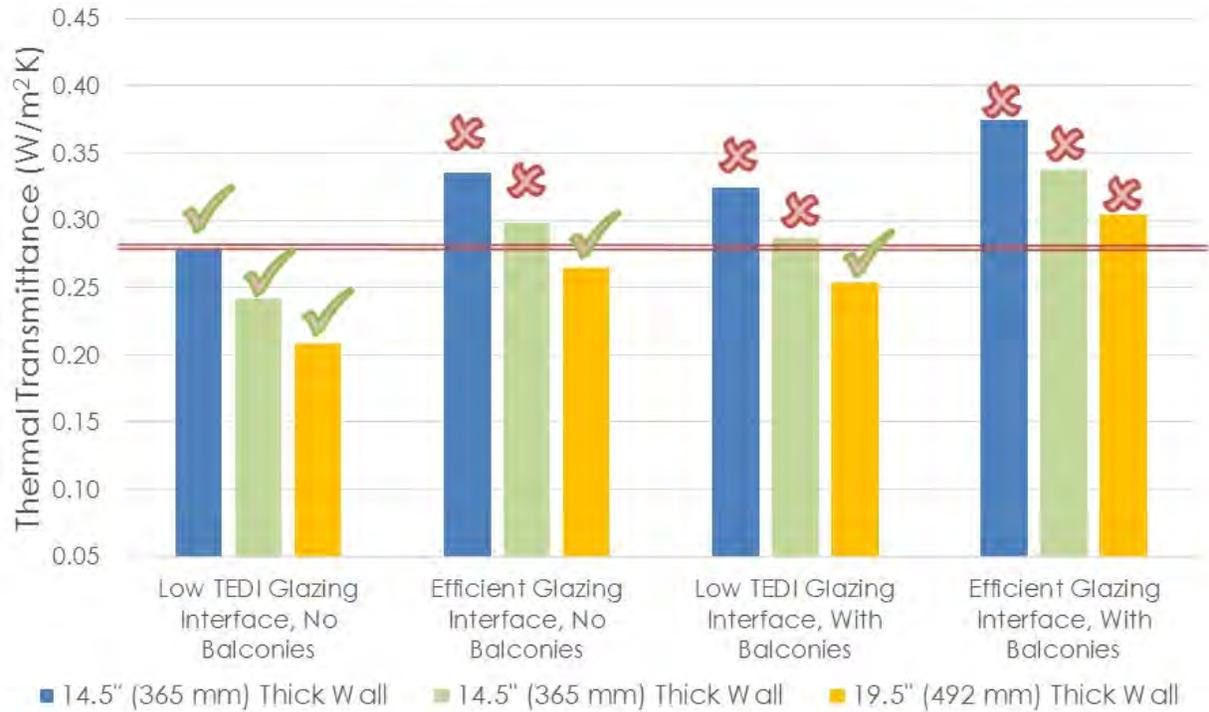
**Figure 6.4:** Impact of Balconies on Wall Thickness for a Target of 0.28 W/m<sup>2</sup>K (R-20 effective) for Low TEDI Glazing Interfaces and R-19 Cavity Insulation Scenarios
