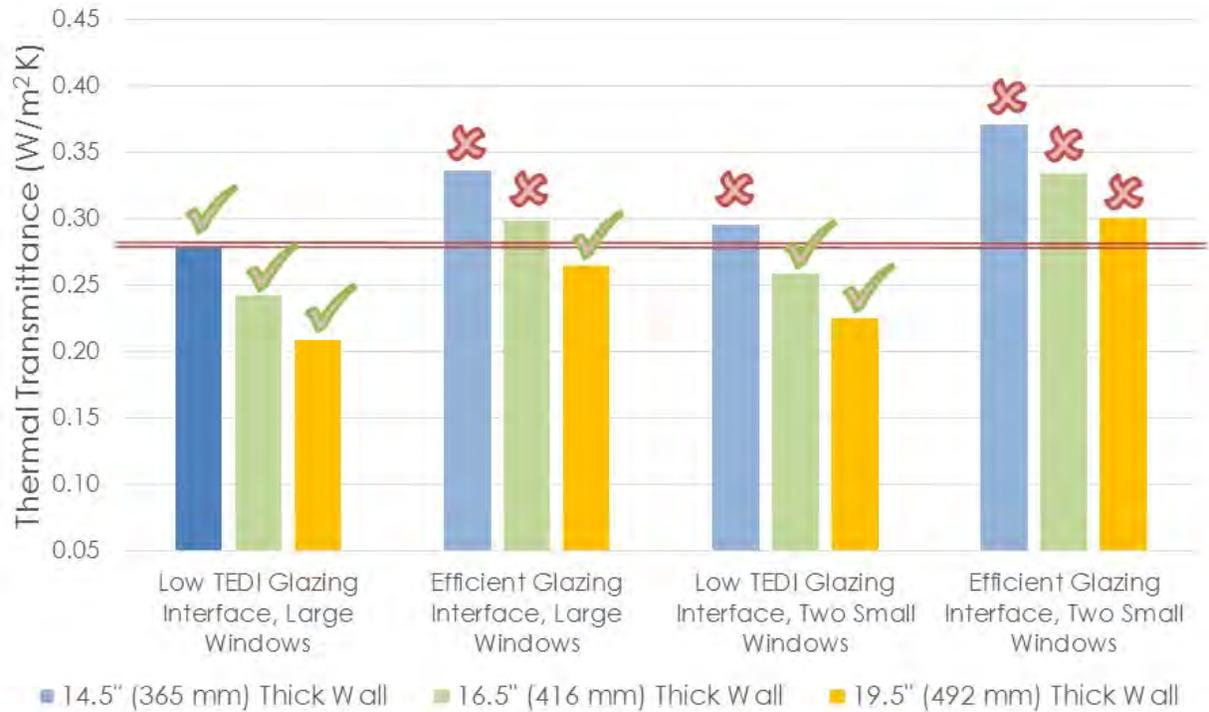
**Figure 6.5:** Impact of Window Size for a Fixed Glazing Ratio on Wall Thickness for a Target of 0.28 W/m<sup>2</sup>K (R-20 effective)
