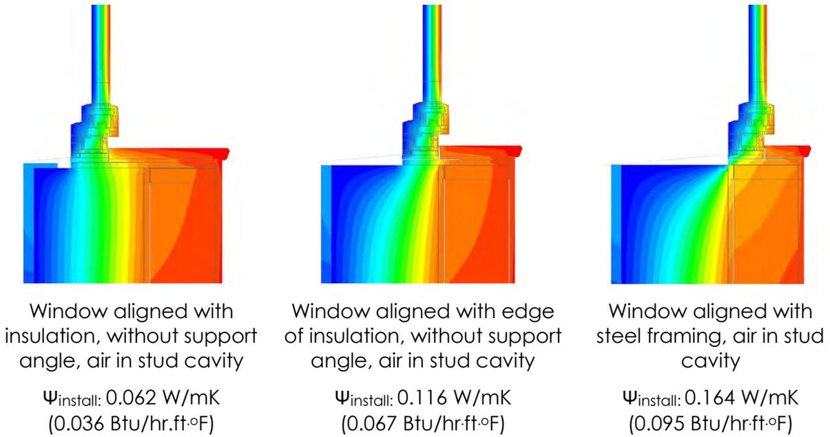
**Figure 5.9:** Impact of Window Positioning on Linear Transmittance
