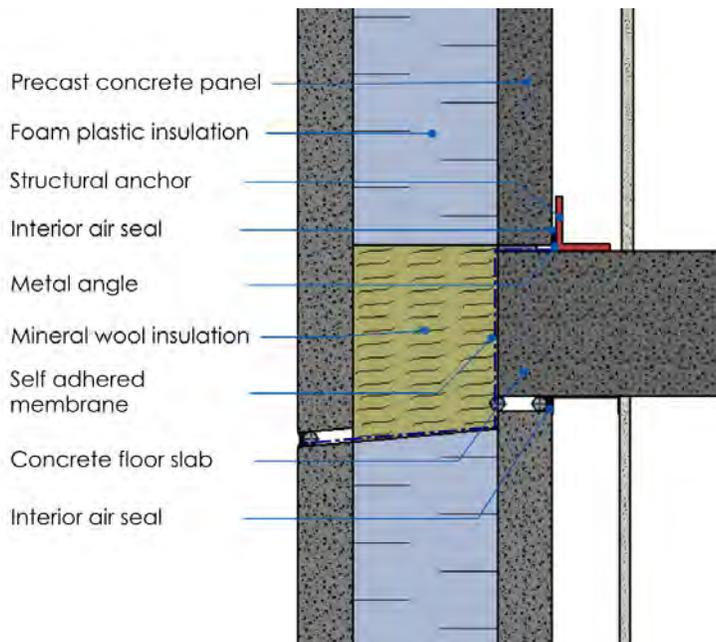
**Figure 5.7:** Example Precast Sandwich Panel with Enhanced Detailing
