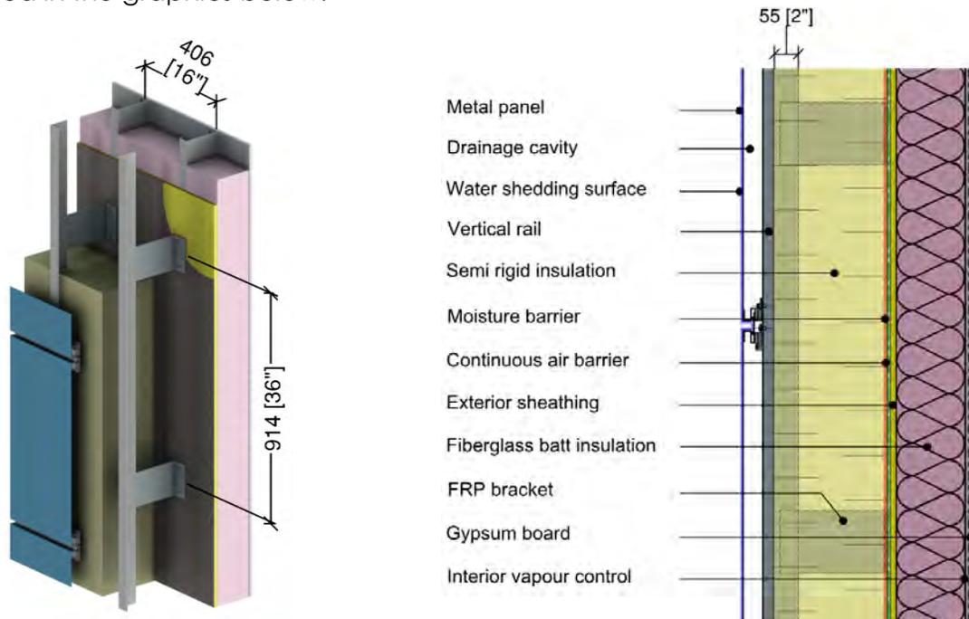
Two scenarios were evaluated, with and without R-19 fiberglass batt insulation in the stud cavity. The results for the clear field wall assembly are presented in **Table 5.2**.
