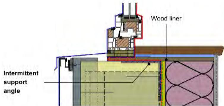
**Figure 5.8:** Support Angle below Window and Wood Liner
