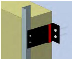
**Type 3 - Glazing Type Thermal Breaks:** Aluminum support brackets have plastic thermal breaks similar to thermally broken windows. The outer metal rail or sub-girt can partially penetrate the insulation or be entirely in the cavity behind the cladding, which may also have a plastic shim between the metal bracket and outer metal rail or sub-girt.
