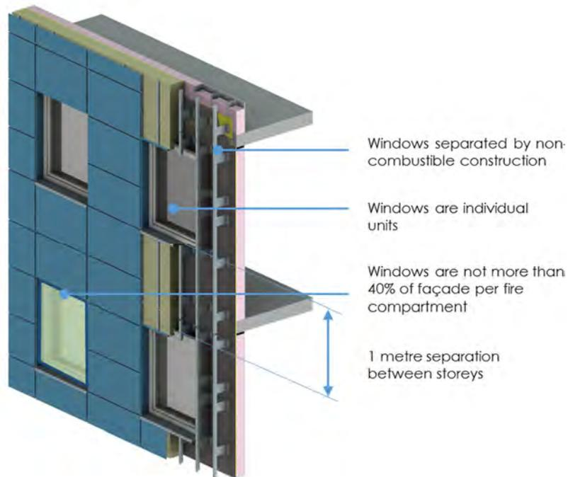
**Figure 5.3:** Combustible Window Frames in Noncombustible Construction
