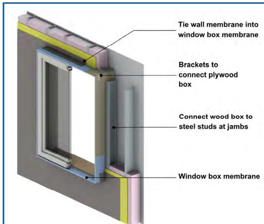
**Figure 5.6:** Detailing of Window with a Wood Box
