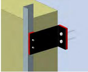
**Type 1 - Shims:** A combustible material functions as a shim, often 5 mm to 20mm (2/5 inches to 3/4 inches) in depth, where metal fasteners connect a metal structural component through to another component. The shims can be buried in the insulation at the sheathing, anywhere in the insulation to connect together two components of the support system, or between the cladding and cladding support system.
