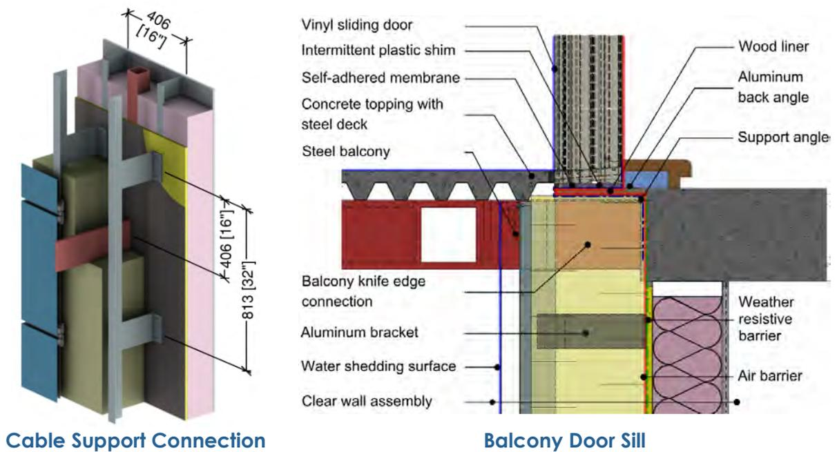
**Table 5.9:** Door with Intermittently Attached Balcony Thermal Transmittances
