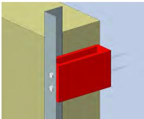
**Type 2 - Thermal Spacers:** The combustible material is larger than shims, is the full depth of the insulation, and functions as a rigid spacer for the connection of long metal fasteners through the insulation back to the structure. The outer rail or sub-girt is completely outboard of the thermal spacer for the metal fasteners to function as the primary structural attachment. This type of system also often requires plastic shims at the sheathing to plumb the cladding.
