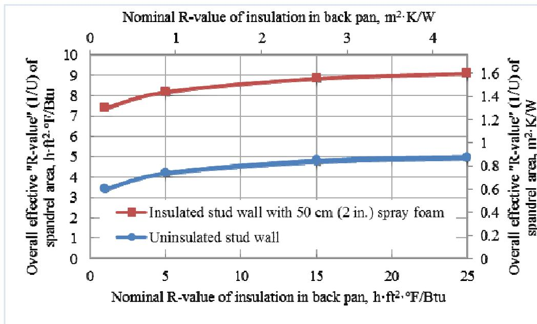
Figure 3. Overall effective “R-value” (1/U) of spandrel areas of curtain wall
