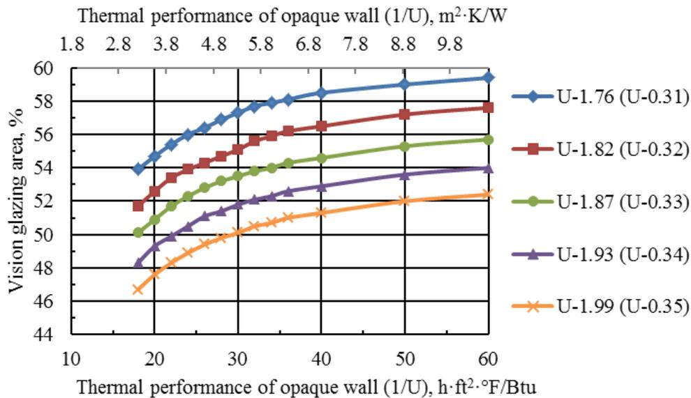
Figure 2. Maximum allowable fenestration area for a given thermal performance of the opaque.
